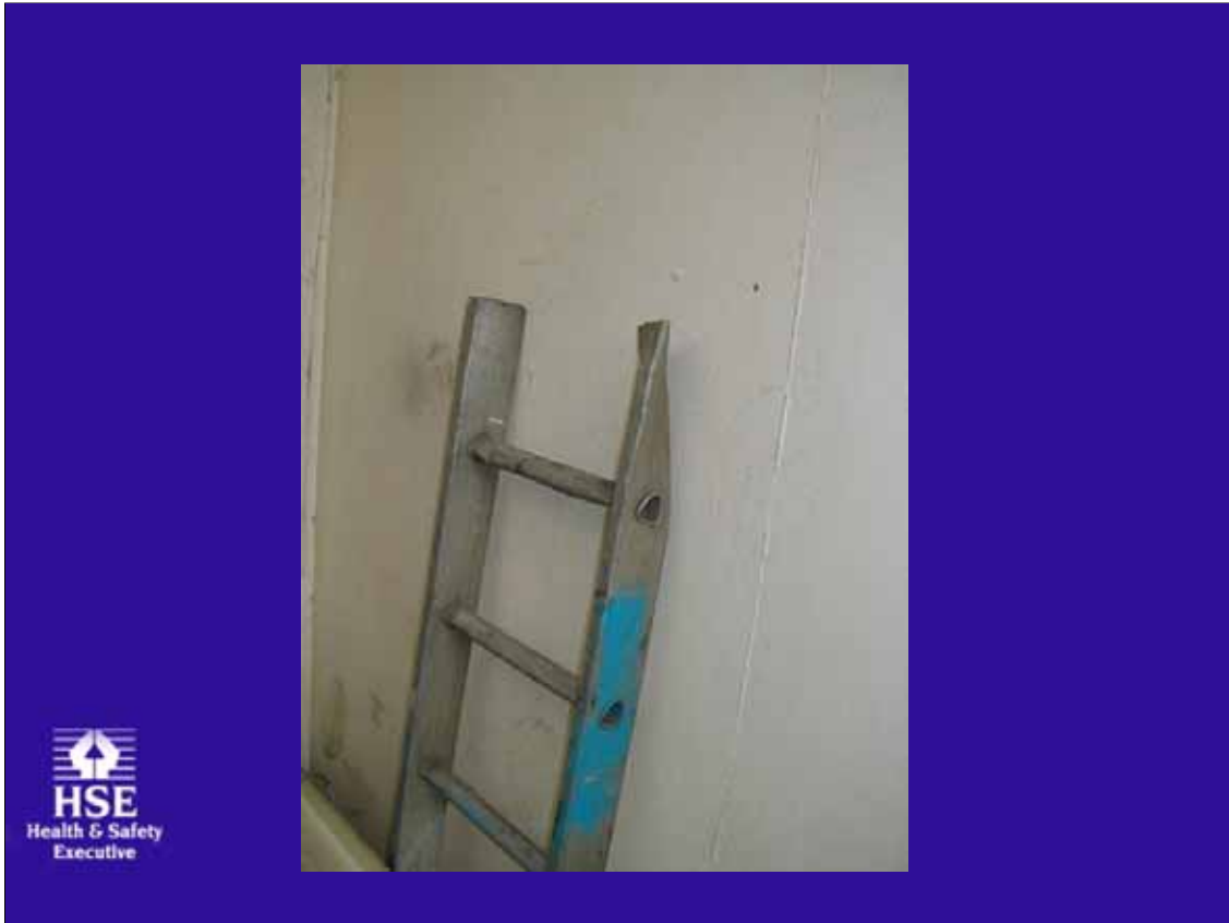
Twisted stile – beyond repair
