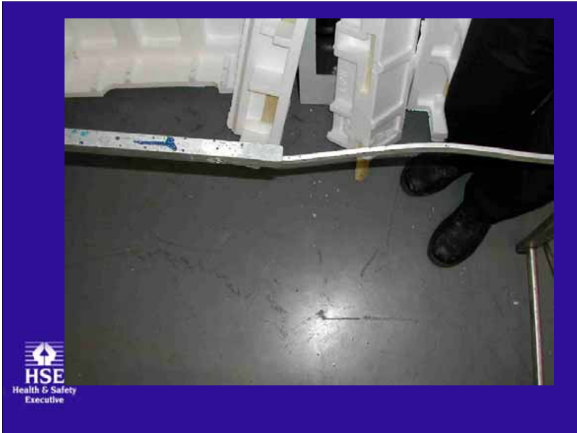
Bent restraint bar – beyond repair
