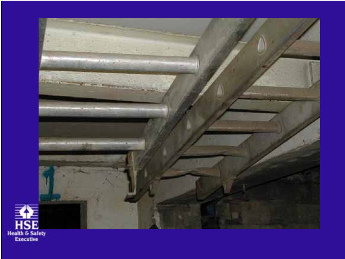
Dented and twisted rungs – beyond repair
